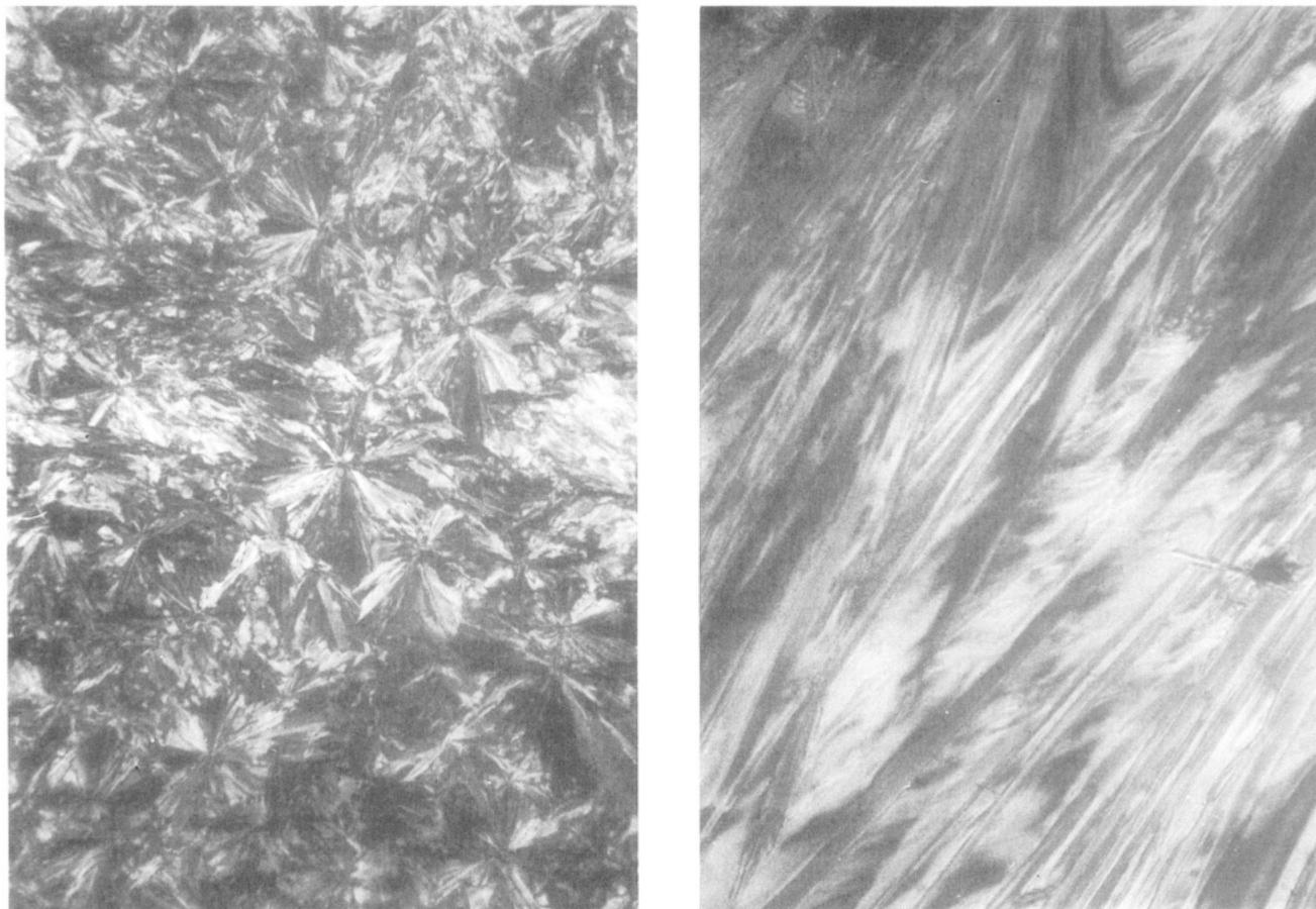
**Figure 3.** Photomicrographs of liquid crystal phases viewed through cross polarizers at 100 $\times$  magnification. Left: ( $\pm$ )-13 heating from solid phase to 74  $^{\circ}$ C. Right: (-)-13 cooling of isotropic melt to 91.1  $^{\circ}$ C.
