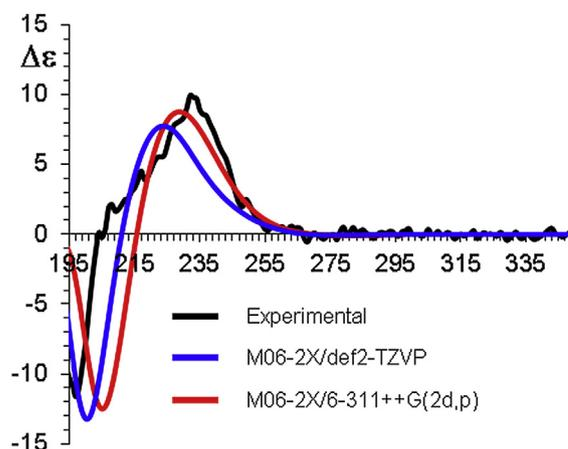
**Fig. 2.** TD-DFT Simulations of the ECD spectrum of **6b** (red and blue traces). The experimental spectrum (black trace) was obtained of acetonitrile solution ( $1.0 \cdot 10^{-4}$  M, 0.2 cm path length).  $\Delta\epsilon$  are expressed in  $\text{mol L}^{-1} \text{cm}^{-1}$ .
