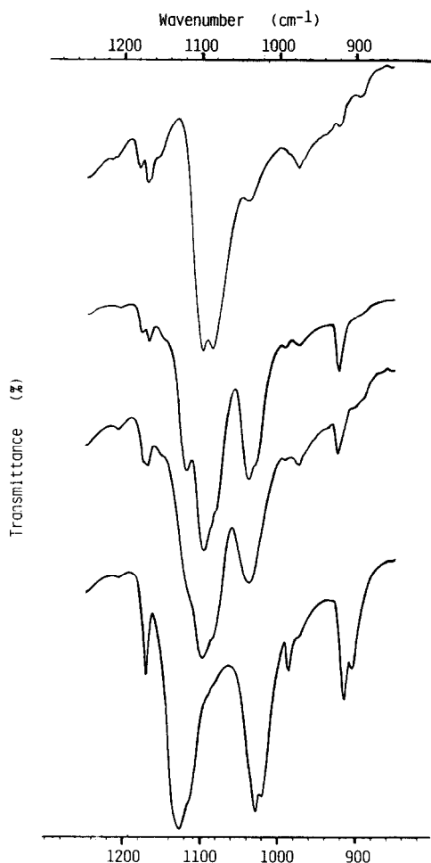
Fig. 3. The \nu(\text{ClO}_4^-) region (nujol/NaCl, 1250–850 \text{cm}^{-1} ) for [\text{Co}(\text{CNR})_5]\text{ClO}_4 \cdot \text{CHCl}_3 , [\text{Co}(\text{CNR})_5]\text{Co}(\text{CNR})(\text{ClO}_4)_2 \cdot 0.5\text{H}_2\text{O} , [\text{Co}(\text{CNR})_5](\text{ClO}_4)_2 \cdot \text{CH}_2\text{Cl}_2 , and [\text{Co}(\text{NCR})_4](\text{ClO}_4)_2 \cdot \text{CH}_2\text{Cl}_2 (top to bottom, respectively), where \text{R} = 2,6\text{-Me}_2\text{C}_6\text{H}_3 .
