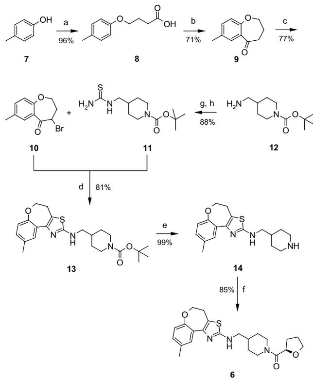
**Scheme 1.** Reagents and conditions: (a) NaOMe,  $\gamma$ -butyrolactone, 1,2-dichlorobenzene, EtOH, 150 °C; (b) PPA, 110 °C; (c) Br<sub>2</sub>, Et<sub>2</sub>O, 25 °C; (d) DIPEA, EtOH, reflux; (e) TFA, CH<sub>2</sub>Cl<sub>2</sub>, 25 °C; (f) (*R*)-(+)-tetrahydro-2-furoic acid, EDC, pyridine, CH<sub>2</sub>Cl<sub>2</sub>, 25 °C; (g) PhCONCS, THF, reflux; (h) K<sub>2</sub>CO<sub>3</sub>, MeOH/H<sub>2</sub>O 3:1, reflux.
