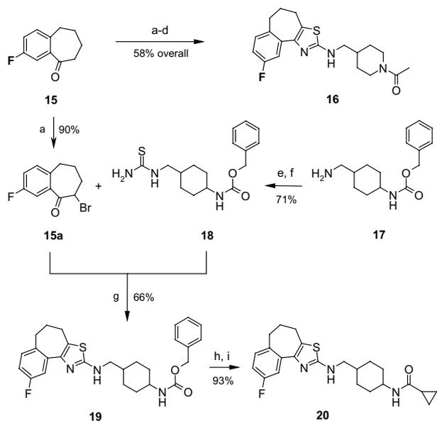
**Scheme 2.** Reagents and conditions: (a)  $\text{Br}_2$ , AcOH, 25 °C; (b) **11**, DIPEA, EtOH, reflux; (c) 5 N HCl in *i*PrOH, 25 °C; (d) acetyl chloride,  $\text{NEt}_3$ ,  $\text{CH}_2\text{Cl}_2$ , 0–25 °C; (e) PhCONCS, THF, reflux; (f)  $\text{K}_2\text{CO}_3$ , MeOH/ $\text{H}_2\text{O}$  3:1, reflux; (g) DIPEA, EtOH, reflux; (h) TMS-I, acetonitrile, 0–25 °C; (i) cyclopropane carboxylic acid chloride,  $\text{NEt}_3$ ,  $\text{CH}_2\text{Cl}_2$ , 0–25 °C.
