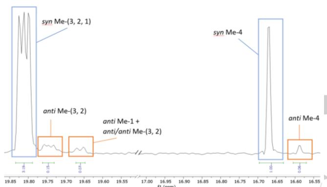
**Figure 3.**  $^{13}\text{C}$ -NMR analysis of compound **21** (note: cut-out 17.05 -19.50 ppm). Resolution enhanced with TRAF apodization.
