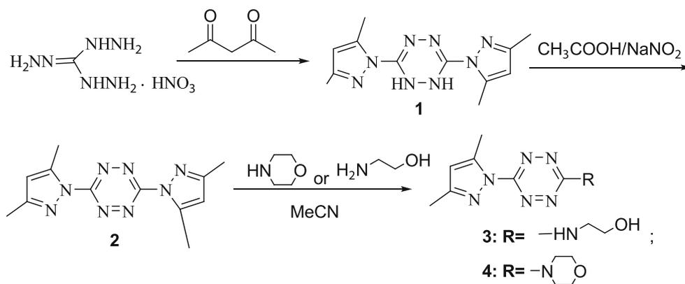
$w = 10\%$ ) was slowly added dropwise aqueous solution of sodium nitrite (100 ml,  $w = 10\%$ ) at 20–30 °C. The reaction mixture was kept at room temperature with continuous stirring for 3 h, then filtered, washed by water (50 ml) and dried to get the red powder (20.5 g, 94.9%).
