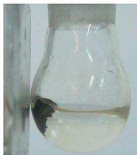
Fig. 5 Photograph showing the magnetic separation of  $\text{Pd@agarose-Fe}_3\text{O}_4$  catalyst from the PEG phase by an external magnet.
