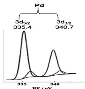
**Fig. 2** X-ray photoelectron spectra of LDH-Pd(0).
