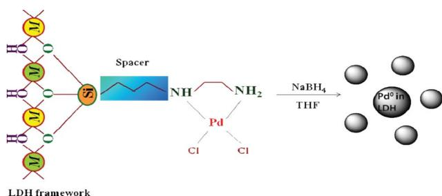
**Scheme 1** Schematic synthesis approach towards Pd<sup>0</sup> nanoparticles.
