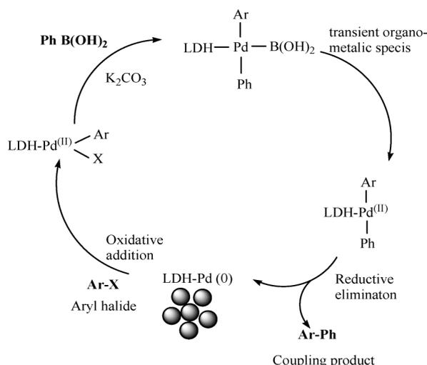
**Scheme 2** Plausible mechanistic pathway for Suzuki coupling.
