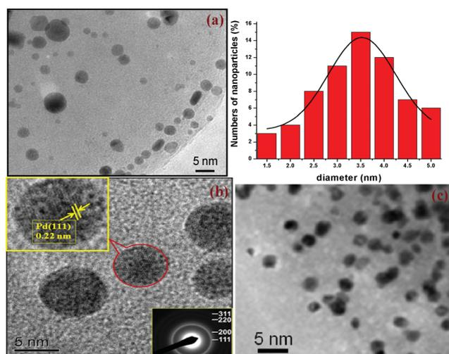
**Fig. 1** (a) TEM image of Pd nanoparticles and histogram showing the size distribution for the Pd nanoparticles. (b) TEM image of Pd nanoparticles with electron diffraction pattern (inset, bottom right). (c) TEM image of the recycled catalyst.
