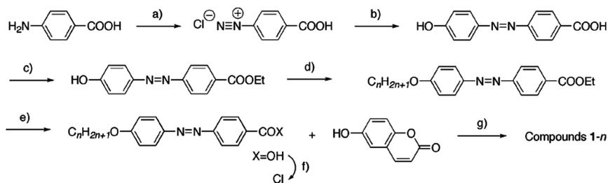
**SCHEME 1** Synthetic scheme for compounds 1-*n*; Reagents and conditions; a) NaNO<sub>2</sub>, 1 M HCl, b) Phenol in 6 M NaOH, then poured into 2 M HCl, c) H<sub>2</sub>SO<sub>4</sub>, EtOH, reflux, d) C<sub>n</sub>H<sub>2n+1</sub>Br, K<sub>2</sub>CO<sub>3</sub>, 3-pentanone, reflux, e) 6 M NaOH, then poured into 2 M HCl, f) SOCl<sub>2</sub> 70°C, g) 6-hydroxycoumarin, pyridine, 70°C.
