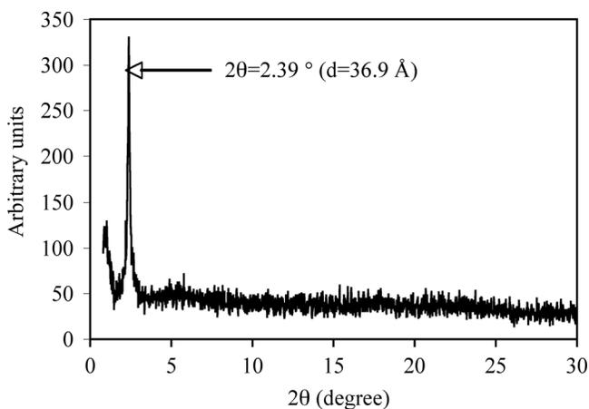
**FIGURE 5** X-ray profile for compound **1-8** at  $160^\circ\text{C}$ .
