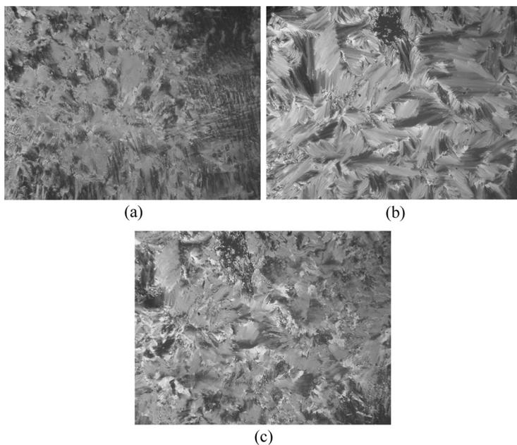
**FIGURE 3** Polarized micrographs for compound 1–8: (a) nematic (N) phase (254°C), (b) smectic A (SmA) phase (202°C), (c) re-entrant nematic (N<sub>re</sub>) phase (132°C).
