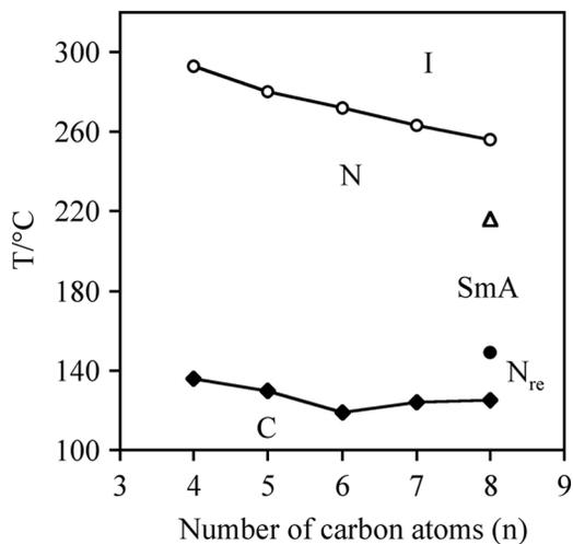
**FIGURE 4** Plots of transition temperatures against the number of the carbon atoms ( $n$ ) for compounds **1-n**; Diamonds, circle (filled), triangle and circles (open) denote melting points,  $N_{re}$ -SmA, SmA-N and N-I transition temperatures, respectively.
