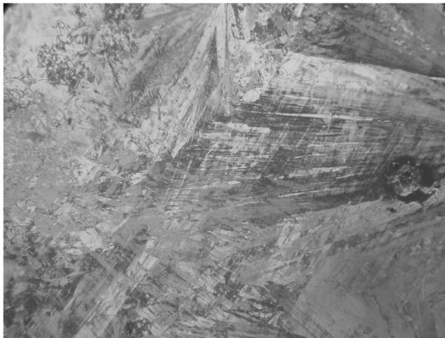
**FIGURE 2** Polarized micrograph for compound 1–7 at 255°C.
