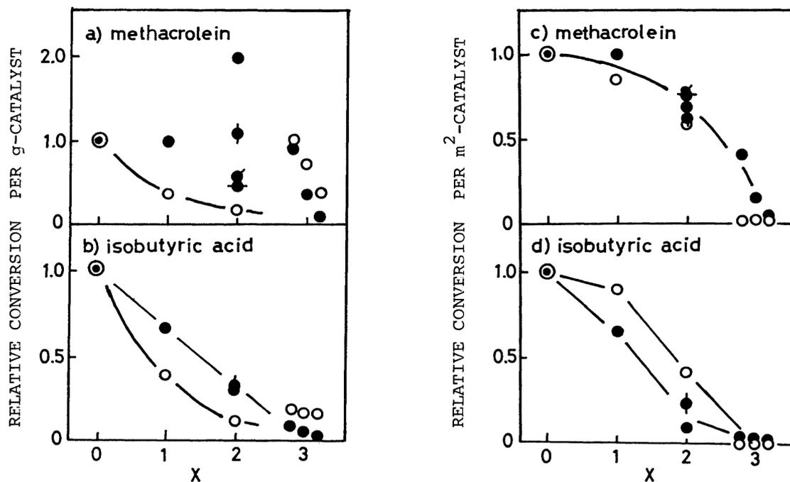
Fig. 1. Relative conversions of methacrolein and methacrylic acid over  $\text{Cs}_x\text{H}_{3-x}\text{PMo}_{12}\text{O}_{40}$  (○) and  $\text{Na}_x\text{H}_{3-x}\text{PMo}_{12}\text{O}_{40}$  (●; flags attached indicate different lots or pretreatments) at 300°C. Conversions over  $\text{H}_3\text{PMo}_{12}\text{O}_{40}$  are taken as 1.0 [Methacrolein(1 μl): 16% over 400 mg-cat., isobutyric acid(1 μl): 75% over 50 mg-cat.].
