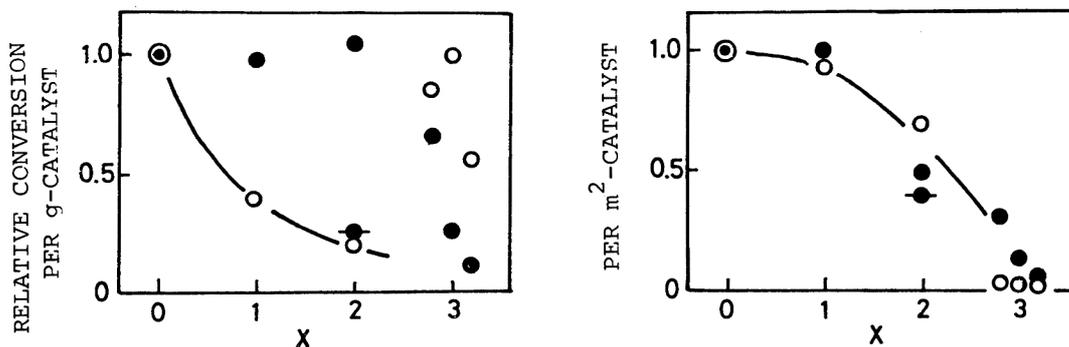
Fig. 2. Relative conversions of acetaldehyde over  $\text{Cs}_x\text{H}_{3-x}\text{PMo}_{12}\text{O}_{40}$  (○) and  $\text{Na}_x\text{H}_{3-x}\text{PMo}_{12}\text{O}_{40}$  (●, ●; different pretreatments) at 300°C.
