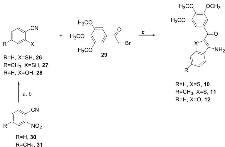
**Scheme 2.** Reagents and conditions: (a) C<sub>6</sub>H<sub>5</sub>CH<sub>2</sub>SH, KOH, DMF; (b) AlCl<sub>3</sub>, C<sub>6</sub>H<sub>6</sub>; (c) K<sub>2</sub>CO<sub>3</sub>, acetone, reflux, 12 h.
