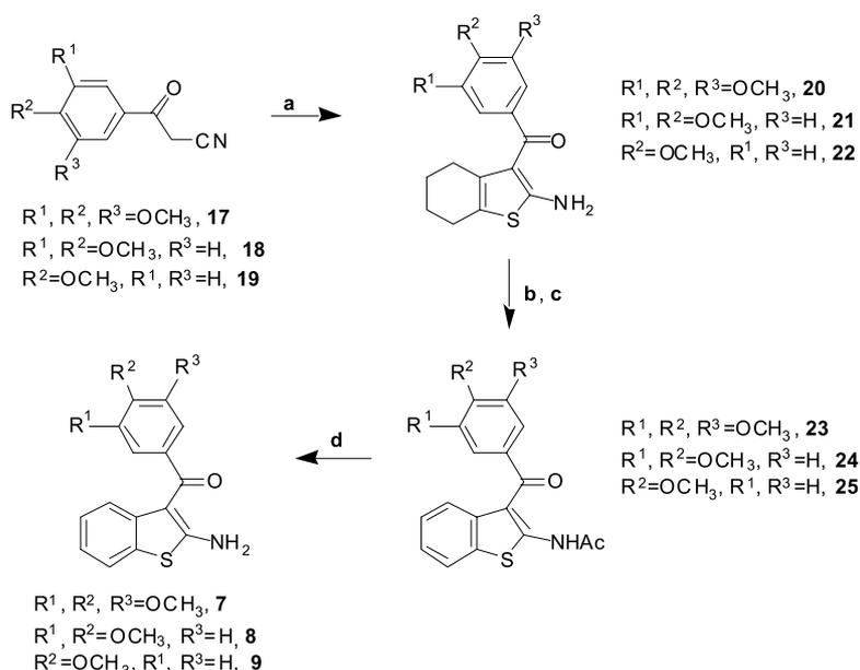
**Scheme 1.** Reagents and conditions: (a) cyclohexanone, S<sub>8</sub>, morpholine, EtOH, 70 °C for 1 h then 18 h at rt; (b) Ac<sub>2</sub>O, pyridine, reflux; (c) 10% Pd/C moistened with a 50% water, 130 °C, 18 h; (d) KOH, EtOH, reflux, 2 h.
