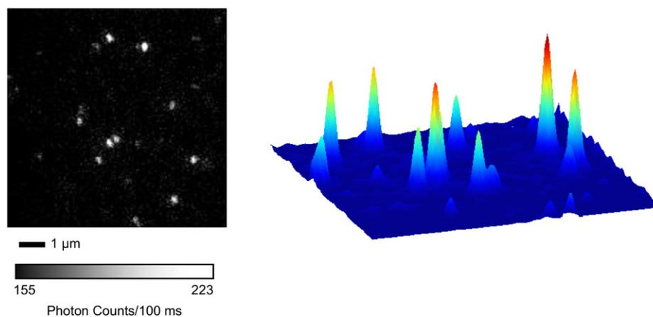
**Figure 2.** Epifluorescence images of single copies of **17** in a PMMA film imaged at 488-nm excitation. The surface was calculated from two position dimensions and pixel intensity of a Gaussian-smoothed image.
