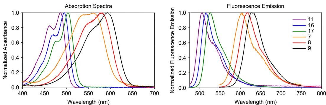
**Figure 1.** Normalized absorption and fluorescence emission spectra for constrained derivatives and their parent molecules. Increasing the constraint on the amine rotation red shifts the absorbance and emission (for structures see Table 1).
