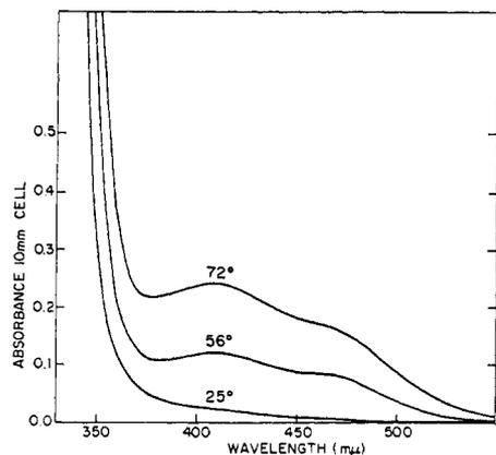
Figure 3. Optical spectra of 0.019  $M$   $\text{Ni}[\text{P}(\text{O}-p\text{-tolyl})_3]_4$  at various temperatures in benzene.
