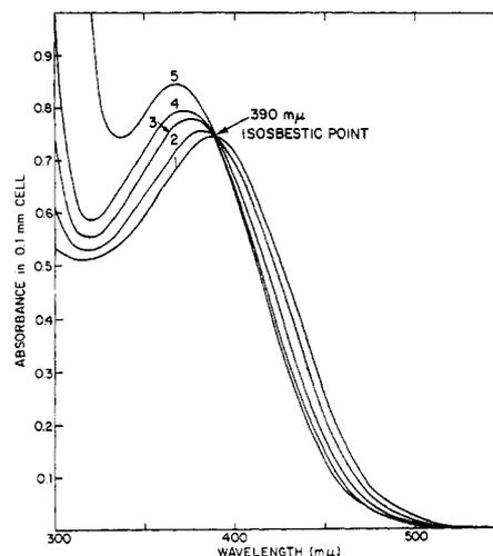
Figure 5. Optical spectra of  $3.64 \times 10^{-3} M$   $\text{Ni}[\text{PMePh}_2]_4$  in benzene at 25° with increasing concentrations of added  $\text{PMePh}_2$ : (1) none; (2) 0.02  $M$ ; (3) 0.05  $M$ ; (4) 0.10  $M$ ; (5) 2.0  $M$ .
