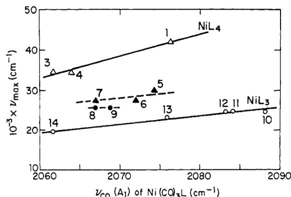
Figure 2. Frequency of longest wavelength electronic absorption maximum vs. A<sub>1</sub> stretching frequency of Ni(CO)<sub>3</sub>L from ref 33: Δ, NiL<sub>4</sub> without P-Ph; ▲, NiL<sub>4</sub> with P-Ph; ●, NiL<sub>3</sub> with P-Ph; ○, NiL<sub>3</sub> without P-Ph. The ligand numbers refer to Table IV.
