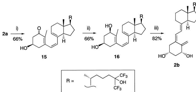
**Scheme 3.** The preparation of 1-epimer **2b** from **2a**. (i) Dess–Martin periodinane, CH<sub>3</sub>CN, rt, 4 h; (ii) NaBH<sub>4</sub>, MeOH, 0 °C, 1.5 h; (iii) acetone, 80 °C, 6 h.
