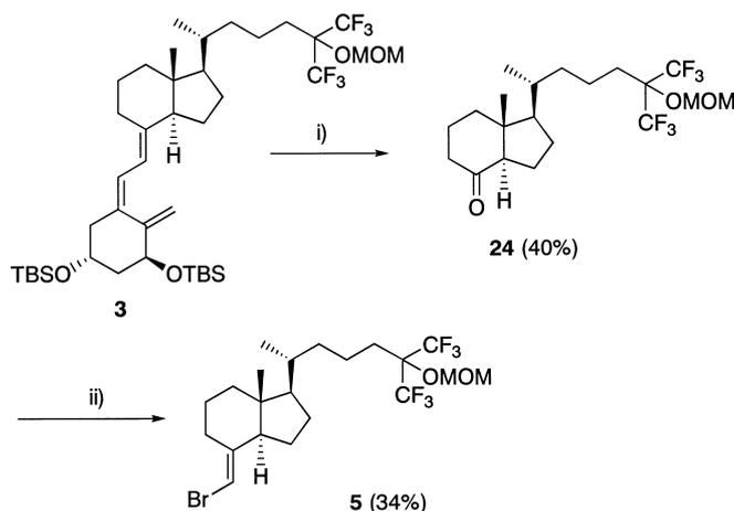
**Scheme 5.** Preparation of the CD ring fragment **5** from **3**. (i)  $\text{O}_3$ ,  $\text{PPh}_3$ ,  $-78^\circ\text{C}$ , 30 min; (ii)  $\text{LiN}(\text{TMS})_2$ , bromotriphenylphosphonium bromide, toluene,  $-78^\circ\text{C}$ , 30 min.
