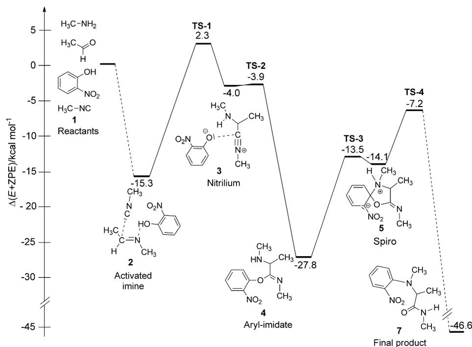
**Scheme 2.** Energy profile of the mechanism of a model Ugi-Smiles reaction. Calculations were carried out at the M06-2X/6-311 + G(d,p) level of theory in toluene.
