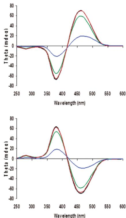
**Figure 3.** Circular dichroism (CD) spectra of L-POWT (top) and D-POWT (bottom) after 30 min of incubation in deionized water (black line), pH 4.0 (red line), pH 5.9 (green line), and pH 10 (blue line).
