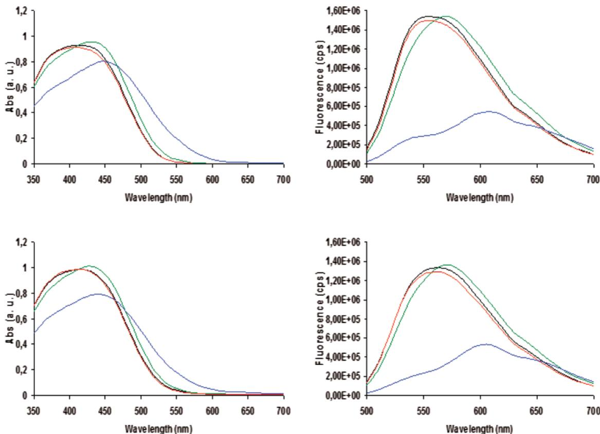
**Figure 2.** Absorption spectra (left) and emission spectra (right) of L-POWT (top) and D-POWT (bottom) after 30 min of incubation in deionized water (black line), pH 4.0 (green line), pH 5.9 (red line), and pH 10 (blue line). All the emission spectra were recorded with excitation at 400 nm.
