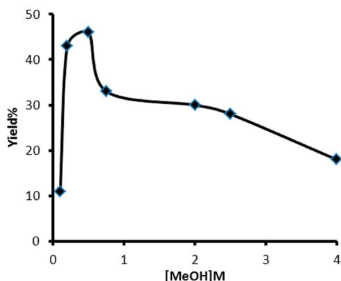
**Figure 3.** Yields in the photostimulated reaction of BN with  $\text{SmI}_2$  as a function of MeOH concentration (see Table 1).
