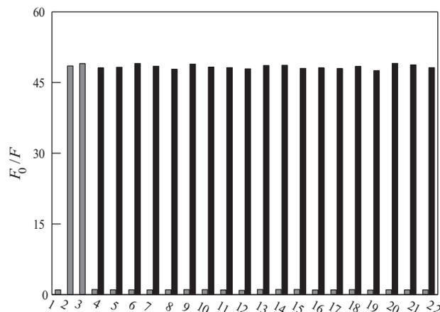
**Fig. 3.** The selectivity of DTI toward various amino acids. Gray bars: the ratio of  $F_0/F$  of DTI in the presence of various amino acids; Black bars: the ratio of  $F_0/F$  of DTI in the presence of the mixture of each amino acid and GSH, (1) Free DTI. (2) Cys. (3) Hcy. (4) Tyr. (5) Gly. (6) Phe. (7) Met. (8) Leu. (9) Arg. (10) Pro. (11) Lys. (12) Glu. (13) Gln. (14) Asp. (15) Iso. (16) Ile. (17) Val. (18) His. (19) Ser. (20) Ala. (21) Thr. (22) Try.
