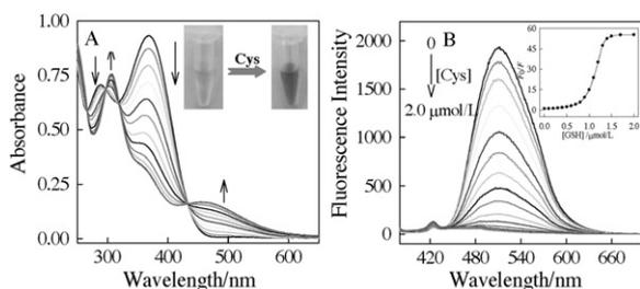
**Fig. 1.** Absorption (A) and fluorescence spectra (B) of DTI in the presence of increasing amounts of Cys in Tris–HCl solution (50 mmol/L, pH 7.4). The arrow indicates the signal changes as increases in Cys concentrations (0, 0.1, 0.2, 0.3, 0.4, 0.5, 0.6, 0.7, 0.8, 0.9, 1.0, 1.1, 1.2, 1.3, 1.4, 1.5, 1.7, 2.0  $\mu\text{mol/L}$ ). Inset: the ratio of  $F_0/F$  of DTI as a function of the concentrations of Cys.
