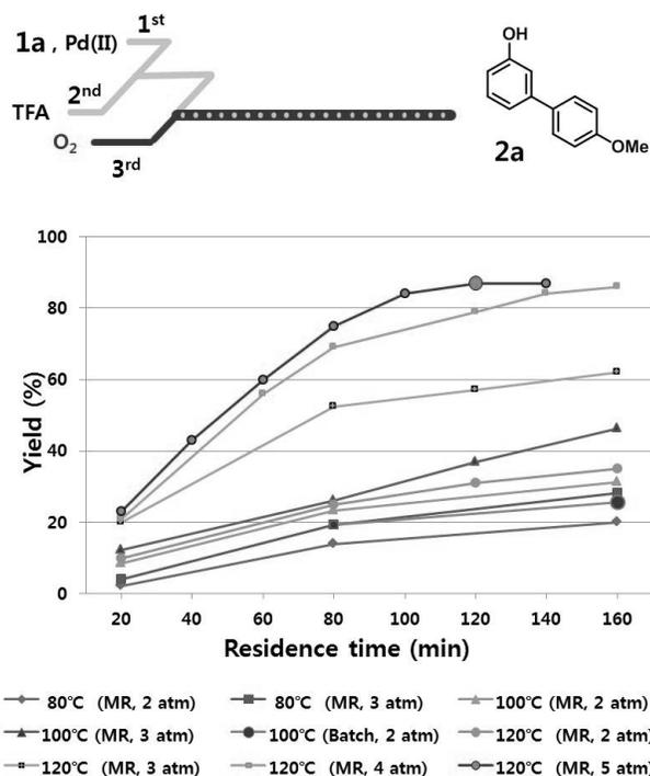
**Figure 5.** Schematic of the microchemical oxidative dehydrogenation. Standard reaction conditions: The reaction solution (0.8 mL) collected from the oxidative Heck reaction in the tube-in-tube microreactor; 5% TFA in DMSO, 2 mL. The overall yield after the first oxidative Heck reaction in the tube-in-tube microreactor and the second oxidative dehydrogenation in the capillary microreactor was determined by <sup>1</sup>H NMR analysis.
