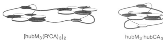
Chart II. Possible Structure for a Dimer of the [1 + 3] Complexes (Left) and a Stable Hydrogen-Bonded [1 + 1] Complex between a Tris Melamine Derivative and a Tris Isocyanuric Acid Derivative (Right)
