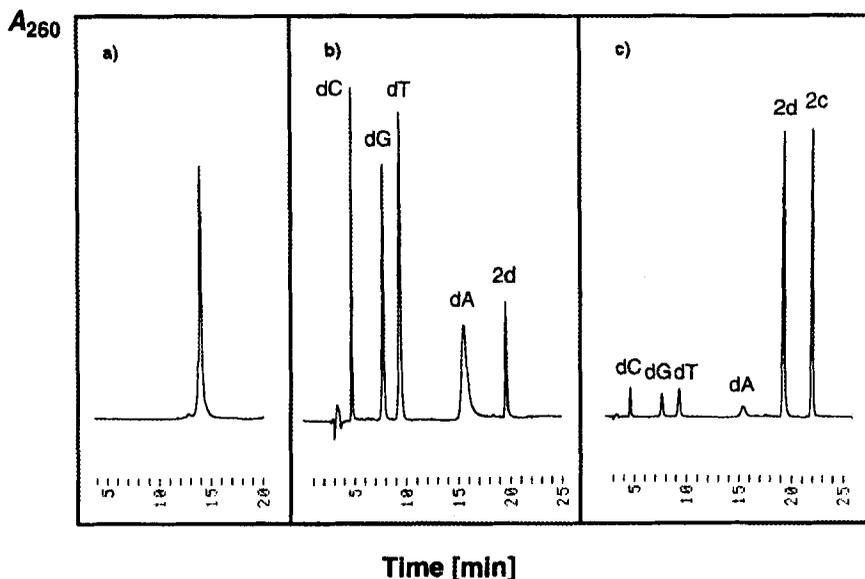
**FIG. 1.** HPLC-Profiles of the oligonucleotide **11**, (a) after oligonucleotide synthesis and work-up, (b) after enzymatic hydrolysis with snake-venom phosphodiesterase followed by alkaline phosphatase in 1M Tris-HCl buffer (pH 8.3), (c) enzymatic digestion in the presence of **2c** and **2d** (c); for a) gradient I, for b) and c) gradient II; details see Exp. Part.
