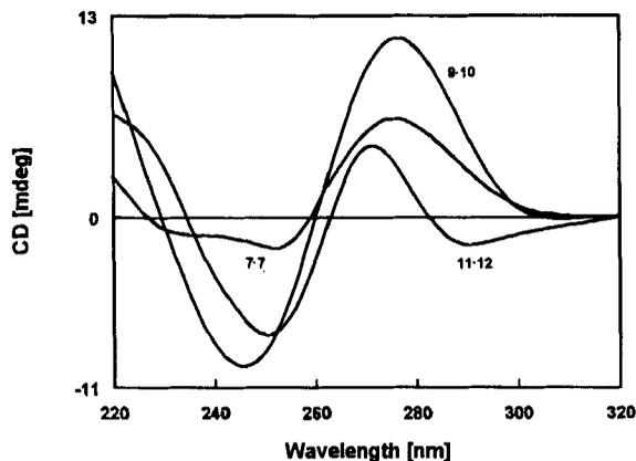
**FIG. 2.** CD spectra of the heteroduplexes **7•7**, **9•10** and **11•12**, measured at 10°C in 1 M NaCl, 100 mM MgCl<sub>2</sub>, and 60 mM Na-cacodylate (pH = 7.0) with 10 μM oligomer concentration; for sequences see Table 3.
