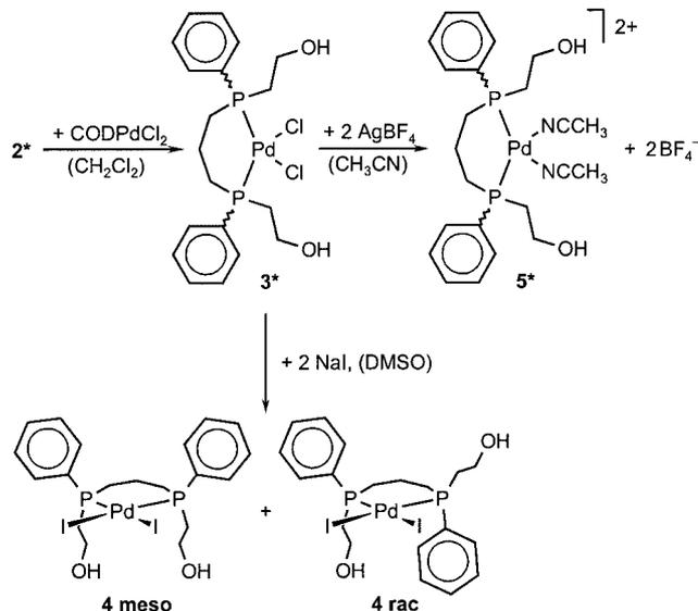
Scheme 3. Preparation of the neutral and dicationic  $\text{Pd}^{\text{II}}$  complexes of ligand **2\***
