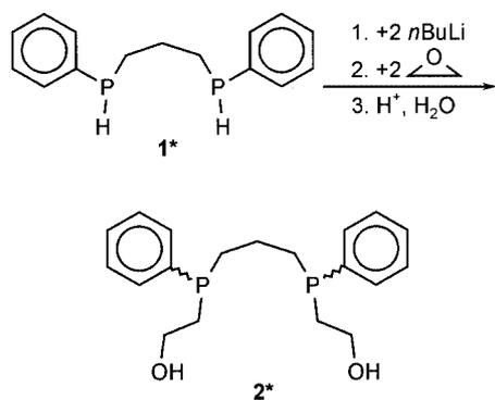
Scheme 2. Synthesis of 2-hydroxyethyl-substituted bisphosphane **2\***
