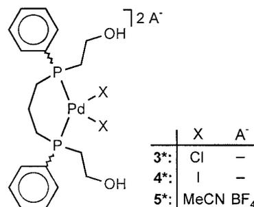
Scheme 1. Novel hydroxy-functionalized bisphosphane Pd<sup>II</sup> complexes
