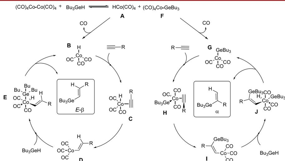
**Figure 3.** Plausible mechanism for the  $Co$ -catalyzed hydrogermylation.
