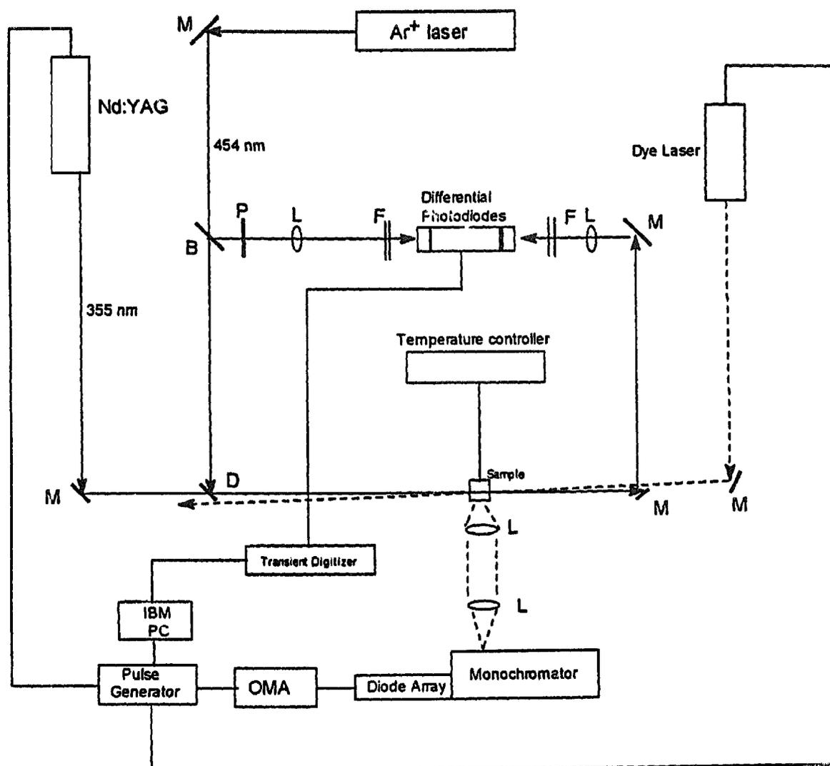
Fig. 2. The experimental setup for the measurements of pulse pump-cw probe transient absorption and pulse pump-pulse probe TSLIF. M: mirror, F: filter, D: dichroic mirror, L: lens, B: beam splitter, P: polarizer, OMA: optical multichannel analyzer.
