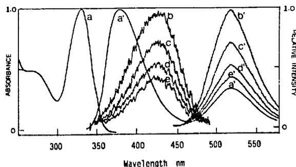
Fig. 3. UV absorption (a) and emission spectra (a') of 7HQ in methanol. Transient absorption ((b)–(e)) and TSLIF ((b')–(e')) of 7HQ in methanol at various delay times between pump (266 nm) and probe pulses (white light pulse for transient absorption, 440 nm dye laser for TSLIF). (b (b')) 200 ns; (c (c')) 1.5  $\mu$ s; (d (d')) 2.5  $\mu$ s; (e (e')) 3.0  $\mu$ s.
