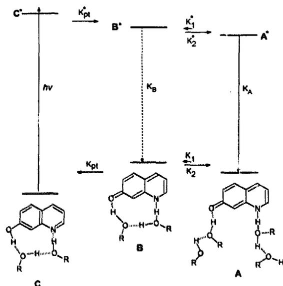
Fig. 1. The proposed proton transfer cycle of 7HQ in alcohol solvents, where A only represents one of the randomly solvated 7HQ. It is noted that Fig. 1 only depicts the complex C of the normal tautomer. Other types of alcohol/normal tautomer complexes in which the ESPT is prohibited during the lifetime of the excited state are not shown.
