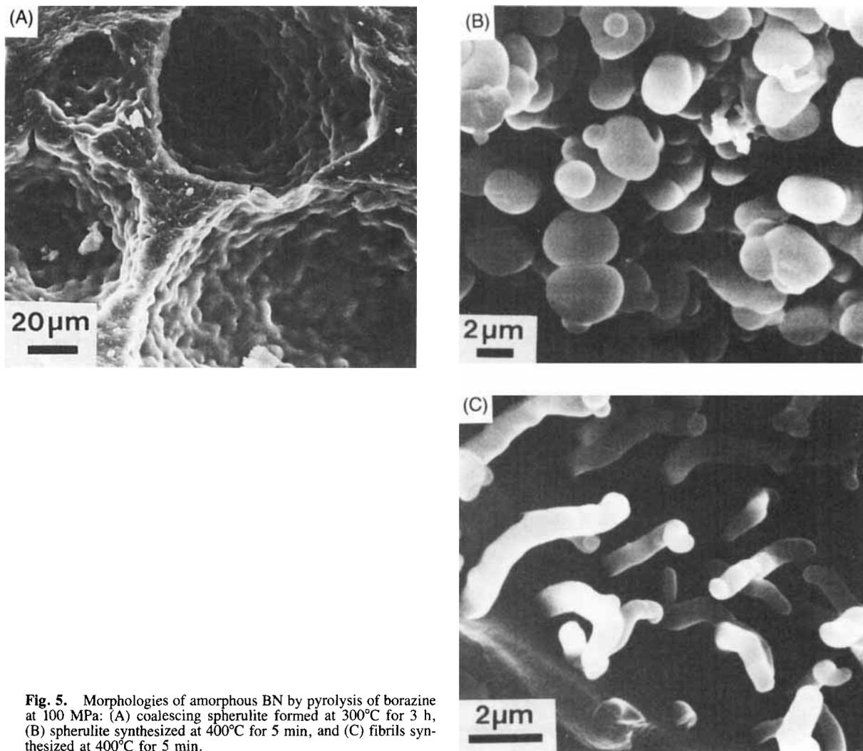
**Fig. 5.** Morphologies of amorphous BN by pyrolysis of borazine at 100 MPa: (A) coalescing spherulite formed at 300°C for 3 h, (B) spherulite synthesized at 400°C for 5 min, and (C) fibrils synthesized at 400°C for 5 min.
