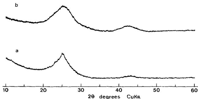
Fig. 1. X-ray diffraction profiles of pyrolysis products of borazine (a) at 250°C and 100 MPa and (b) at 700°C and 100 MPa.
