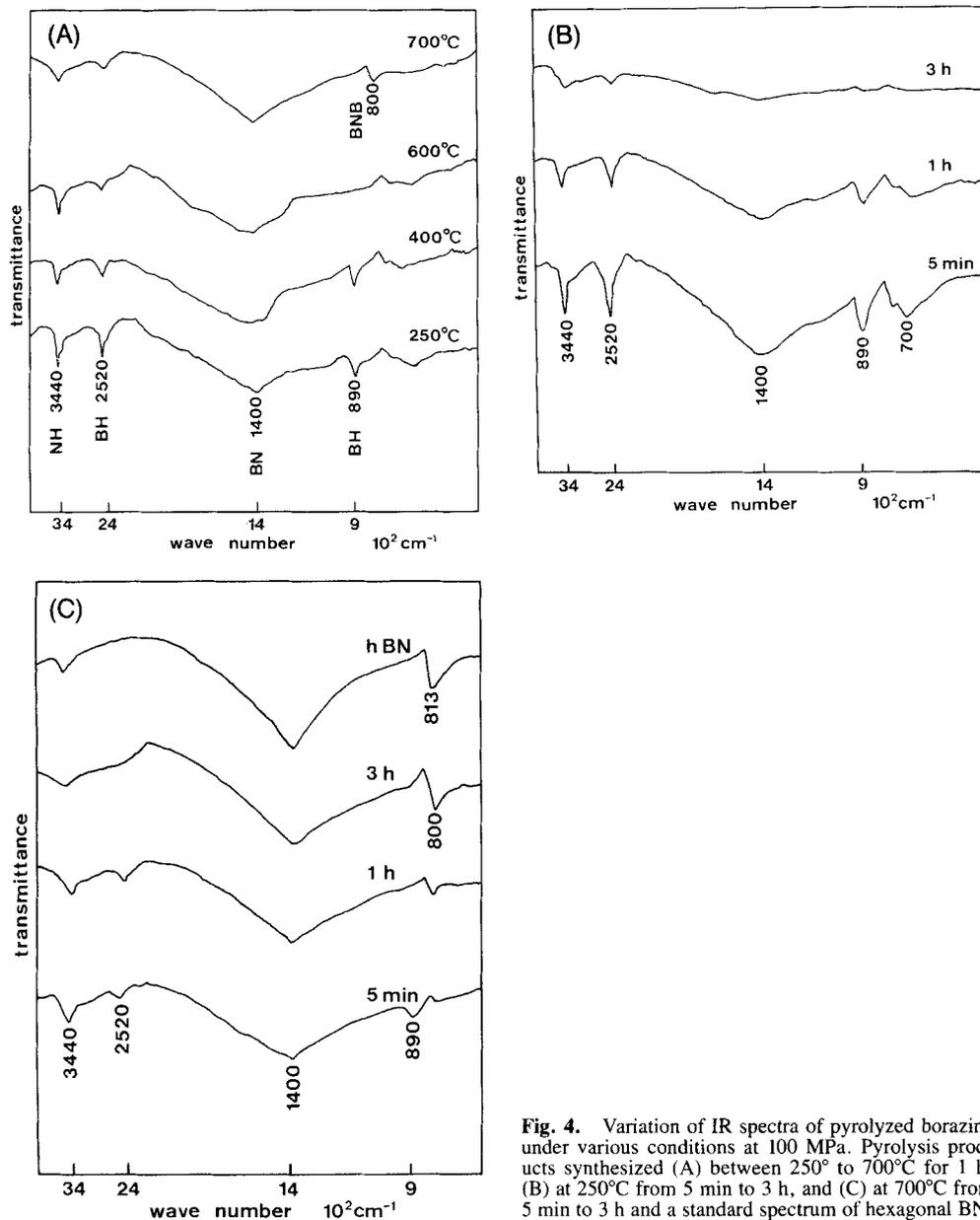
Fig. 4. Variation of IR spectra of pyrolyzed borazine under various conditions at 100 MPa. Pyrolysis products synthesized (A) between 250° to 700°C for 1 h, (B) at 250°C from 5 min to 3 h, and (C) at 700°C from 5 min to 3 h and a standard spectrum of hexagonal BN.
