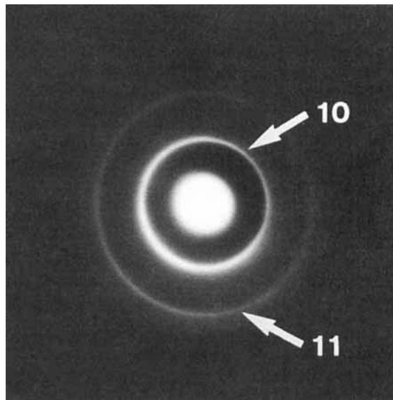
Fig. 2. Selected area diffraction of BN formed from borazine at 600°C and 100 MPa for 3 h.
