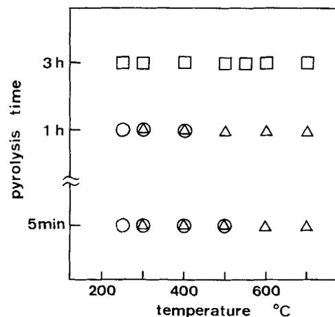
**Fig. 6.** Pyrolysis conditions of borazine and morphology of amorphous BN: (□) coalescing spherulite, (○) spherulite, and (△) fibril.
