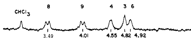
Fig. 3.—The n.m.r. spectrum of 1,2,5,7-tetramethylcyclohepta[ d,e ]-1-pyridine relative to internal tetramethylsilane (TMS = 10.0).
