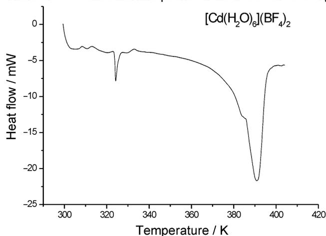
Fig. 1 DSC curve obtained for  $[\text{Cd}(\text{H}_2\text{O})_6](\text{BF}_4)_2$  at a constant heating rate of 10 K min<sup>-1</sup>
