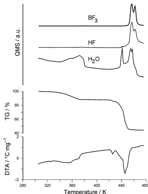
**Fig. 2** DTA, TG and QMS curves obtained for  $[\text{Cd}(\text{H}_2\text{O})_6](\text{BF}_4)_2$  at a constant heating rate of  $2 \text{ K min}^{-1}$  in the flow of air
