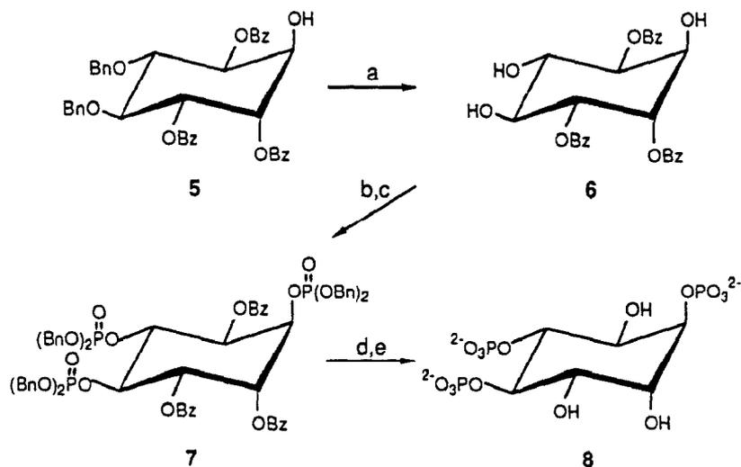
Scheme 2. Pathway for the synthesis of **8**. The reagents are the same as in the legend of Scheme 1.
