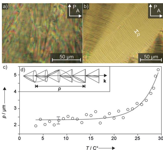
**Figure 6.** a) Pitch lines of a sample with 59 wt% water at 36°C and b) of a sample with 32 wt% formamide at 30°C. c) Pitch values of the latter sample derived directly from the texture images plotted against temperature and d) model of the SmC\* phase illustrating the helical distortion of the tilt direction.
