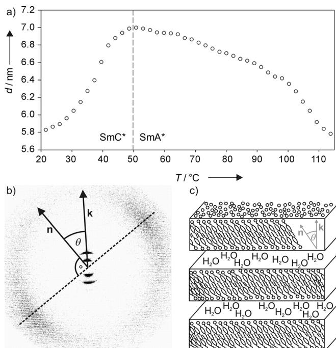
**Figure 5.** a) Temperature-dependent layer spacing  $d$  across the lyotropic  $SmA^*$ - $SmC^*$  transition (64 wt % water), b) 2D diffraction pattern of a monodomain  $SmC^*$  sample (42 wt % water, 38 °C), and c) schematic image of the lyotropic  $SmC$  phase.
