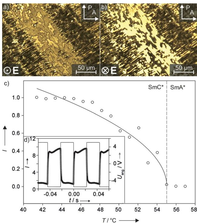
**Figure 7.** The lyotropic SmC\* phase under the influence of an electric field. a) and b) show texture images with reversed directions of an applied electric field with  $U = 5 \text{ V}\mu\text{m}^{-1}$  and  $f = 0.5 \text{ Hz}$  (18 wt% formamide, 25°C). c) Temperature dependence of the change of transmitted light intensity of a sample with 64 wt% water and d) exemplary transmission change (○) at 44°C together with the applied square-wave voltage (—).
