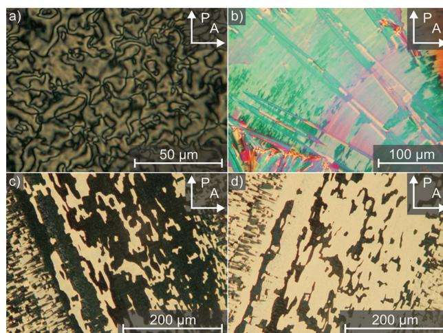
**Figure 4.** Texture images between crossed polarizers (P, A) of the lyotropic  $SmC^*$  phase showing a) a schlieren texture (42 wt % water, 60 °C), b) a broken fan texture with zigzag defect lines (65 wt % water, 46 °C), c) and d) domains with opposite tilt directions in the surface-stabilized state of a 1.6  $\mu m$  cell (17 wt % formamide, 28 °C).
