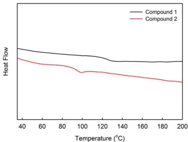
Figure 2. DSC curves of Compound 1 and 2.
