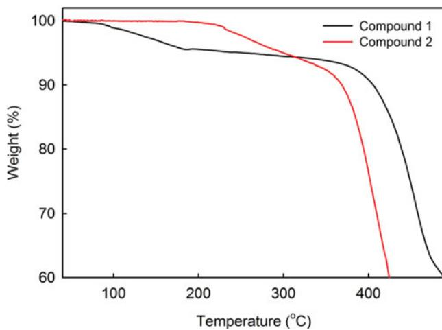
Figure 1. TGA curves of Compound 1 and 2.
