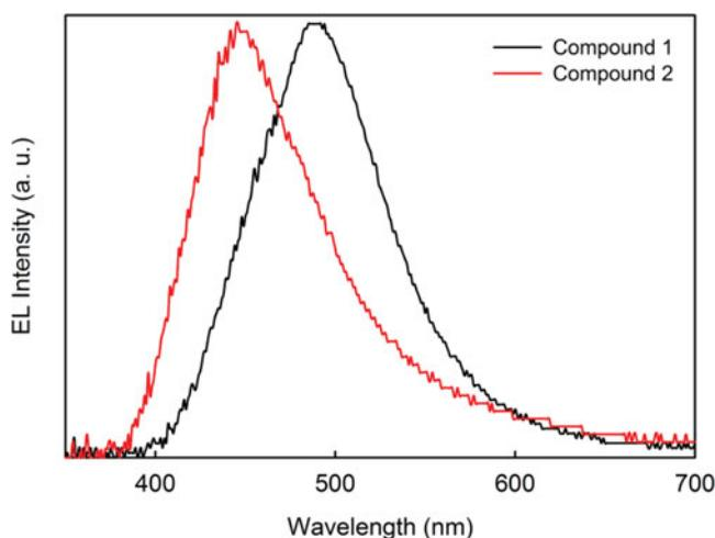
Figure 5. Electroluminescence spectra of compounds 1 and 2.
