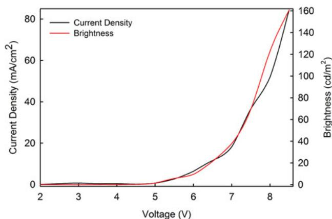
**Figure 7.** Current density-voltage-luminescence (J-V-L) characteristics of compound 1.
