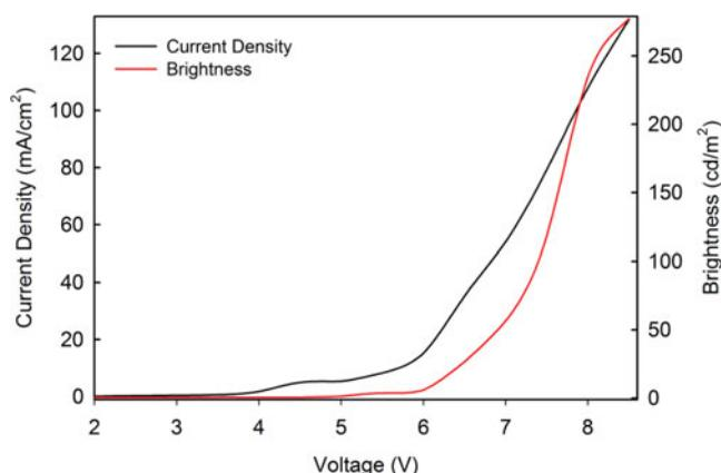
**Figure 6.** Current density-voltage-luminescence (J-V-L) characteristics of compound 1.
