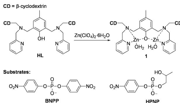
Scheme 1 Synthesis of catalyst **1** and the phosphate diester substrates used in this study.
