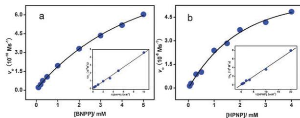
**Fig. 3** Saturation kinetics catalyzed by 0.1 mM **1** in buffer (50 mM TAPS and HEPES), *I* = 0.1 M (NaClO<sub>4</sub>) at 308 ± 0.1 K: (a) **BNPP** hydrolysis at pH 8.82; (b) **HPNP** transesterification at pH 7.95.
