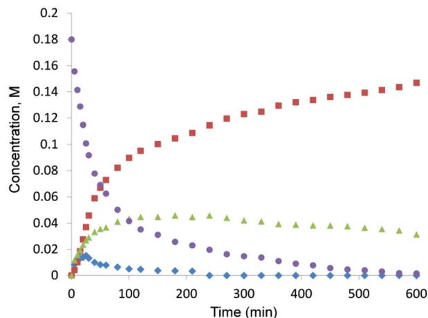
**Fig. 10** Concentration–time plots for B-containing products of dehydrogenation using 2.5 mol% **10** and 0.18 M  $\text{HMe}_2\text{NBH}_3$ . Key:  $\text{HMe}_2\text{NBH}_3$  (circles),  $\text{Me}_2\text{NBH}_2$  (diamonds),  $[\text{Me}_2\text{NBH}_2]_2$  (squares),  $\text{HMe}_2\text{NBH}_2\text{NMe}_2\text{BH}_3$  (triangles).
