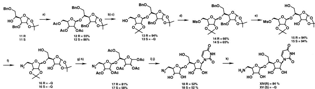
**Scheme 4.** (a) **2**, Hg(CN)<sub>2</sub>, CH<sub>2</sub>Cl<sub>2</sub>, MS 4 Å, rt; (b) MeONa, MeOH, rt; (c) 2-methoxypropene, PTSA, acetone, rt; (d) MsCl, TEA, CH<sub>2</sub>Cl<sub>2</sub>, rt; (e) Pd/C, H<sub>2</sub>, MeOH, rt; (f) NaN<sub>3</sub>, DMF, 70 °C; (g) 60% AcOH aq. 70 °C; (h) Ac<sub>2</sub>O, Pyr., rt; (i) *O,O'*-bis(trimethylsilyl)uracil, TMSOTf, CH<sub>3</sub>CN, rt; (j) MeONa, MeOH, rt; (k) PPh<sub>3</sub>, H<sub>2</sub>O, THF, rt.
