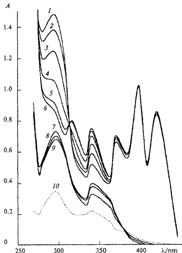
**Fig. 2.** Changes in the UV absorption spectra in the direct photolysis of azide **4** (curves 7–10) and that sensitized by 9-aminoacridine (curves 1–6) under illumination with visible light  $> 400$  nm in methanol; the concentrations of 9-aminoacridine and azide are  $10^{-4}$  mol L<sup>-1</sup>. Time of illumination (min): 0 (1, 7); 5 (2); 15 (3); 30 (4, 8); 60 (5, 9); 600 (6, 10).
