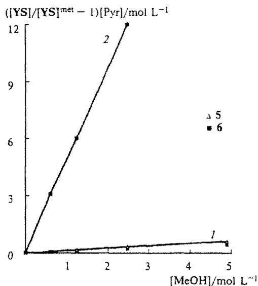
**Fig. 1.** Dependence of  $([YS]/[YS]^{met} - 1) \cdot [Pyr]$  in the photolysis of perfluoroaromatic azides (straight line **1**) and azide **4** (straight line **2**) in a 9.3 M solution of pyridine in heptane on the concentration of methanol.  $[YS]$  and  $[YS]^{met}$  are concentrations of the ylide formed in the absence and in the presence of methanol.
