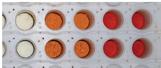
**Fig. 2.** Resin **2** with different loadings in the Vanguard synthesizer (AdvancedChemTech, Ares Block). Resins were not exhaustively dried.
