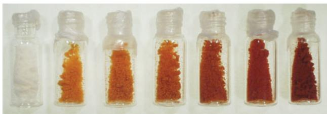
**Fig. 1.** Prepared test row with increasing loading level. Loading level begins on the left side (0 up to 0.93 mmol g<sup>-1</sup>). Resins dried from THF.
