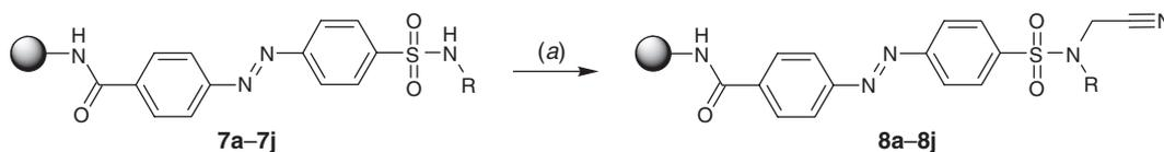
**Scheme 5.** Activation of the polymer-bound carboxylic acid building blocks **7a–7j** with bromoacetonitrile: (a) DIPEA, NMP, bromoacetonitrile.
