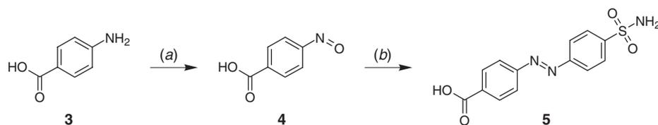
**Scheme 2.** Synthetic pathway towards 4-(4-sulfamoylphenylazo)benzoic acid **5**: (a) H<sub>2</sub>O<sub>2</sub>, Na<sub>2</sub>WO<sub>4</sub>, Bu<sub>4</sub>N<sup>+</sup>Br<sup>-</sup>, H<sub>3</sub>PO<sub>4</sub>, 35–40°C, 3 h; (b) sulfanilamide, acetic acid, 110–120°C, 4 h.
