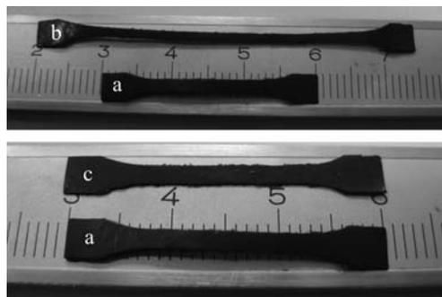
Fig. 3 azoPU (sample A) showing shape memory effect at 75 °C: (a) initial state; (b) deformed state (stretched at 75 °C and fixed at 25 °C); (c) recovered state after heating in oven at 75 °C.
