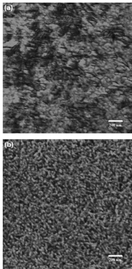
**Fig. 5** AFM phase image for azoPU film spin-coated on a silicon wafer: films prior to UV irradiation (a) and the same film after UV irradiation (254 nm) (b).
