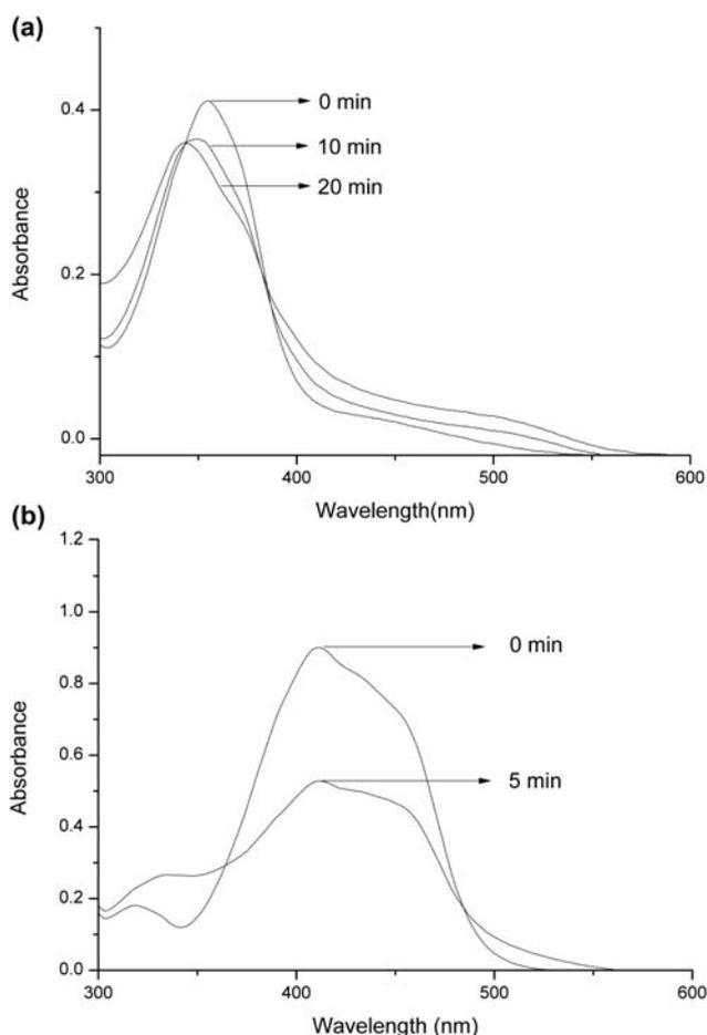
**Fig. 4** UV-vis spectra of azoPU (sample A) with UV irradiation at 254 nm, in chloroform solution (a) and film sample (b).
