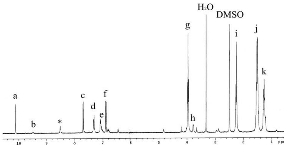
Fig. 2  $^1\text{H}$  NMR spectrum of azoPU (sample A) in  $\text{DMSO-d}_6$  (signal \* existed also in the  $^1\text{H}$  NMR spectrum of pure MDI).<sup>34</sup>
