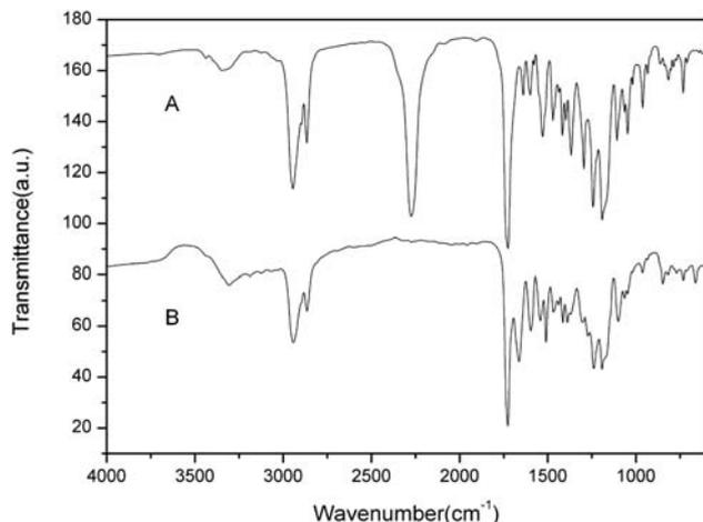
Fig. 1 FTIR spectrum of prepolymer azoPU (A) and sample A (B).
