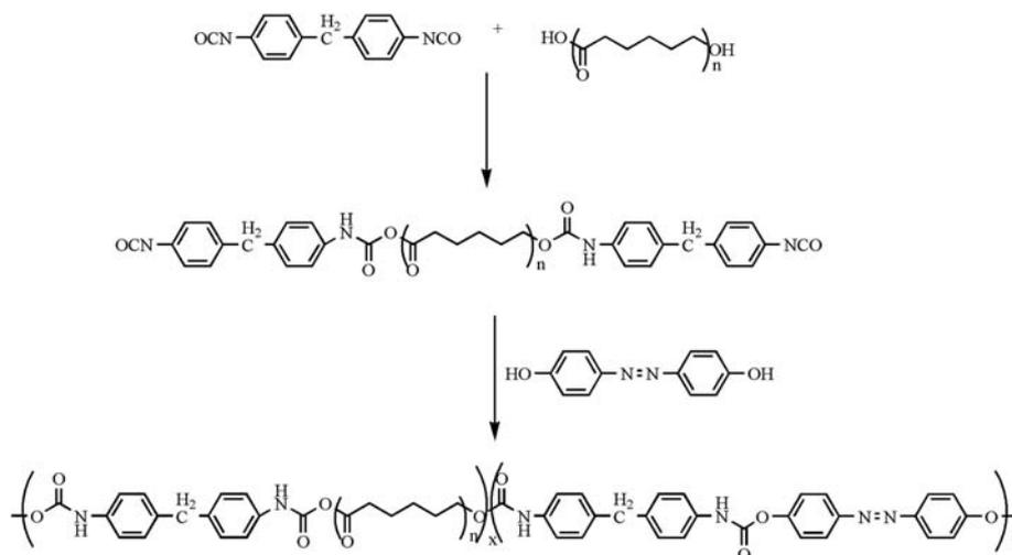
**Scheme 1** Synthetic procedure for SMPU.
