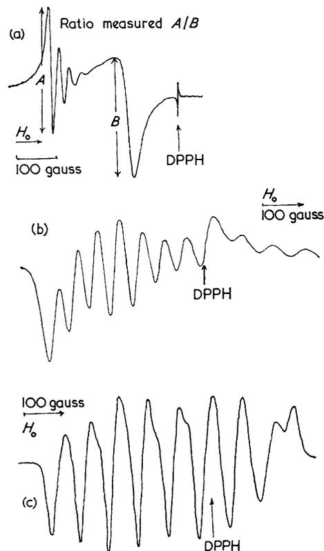
FIGURE 2 E.s.r. spectra (a) the yellow form of  $\text{Co}(\text{CNPh})_5^{2+}$  in  $\text{CH}_2\text{Cl}_2$  after 3 days ( $X$ -band); (b)  $\text{Co}(\text{CNet})_5^{2+}$  in  $\text{CH}_2\text{Cl}_2$  glass at  $77^\circ\text{K}$  ( $X$ -band), characteristic of all the five-co-ordinate isonitrile complexes; (c)  $\text{Co}(\text{CNPh})_5(\text{H}_2\text{O})^{2+}$  in wet  $\text{CH}_2\text{Cl}_2$  at  $77^\circ\text{K}$  ( $X$ -band), characteristic of all the six-co-ordinate complexes
