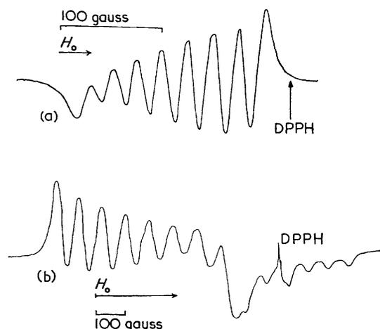
FIGURE 1 E.s.r. spectra of (a)  $\text{Co}(\text{CNEt})_6^{2+}$  in  $\text{CNEt}$  at  $293^\circ\text{K}$  ( $X$ -band); (b)  $\text{Co}(\text{CNEt})_6^{2+}$  in  $\text{CNEt}$  glass at  $150^\circ\text{K}$  ( $Q$ -band)
