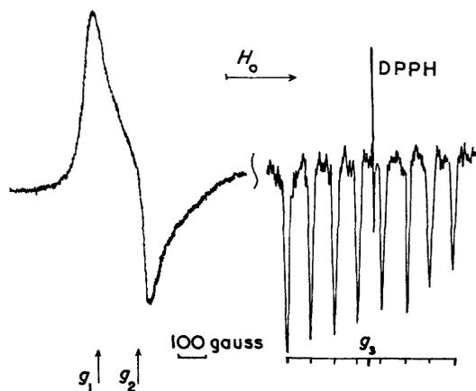
FIGURE 4 E.s.r. spectra of  $\text{Na}_3\text{Co}(\text{CN})_5$  in methanol at  $150^\circ\text{K}$  ( $Q$ -band)
