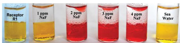
**Figure 10.** Extraction process of  $F^-$  ions from aqueous solutions and seawater using receptor **R1** solution in  $CH_2Cl_2$ .
