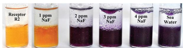
**Figure 8.** Extraction process of  $F^-$  ions from aqueous solutions and seawater using receptor **R2** solution in  $CH_2Cl_2$ .
