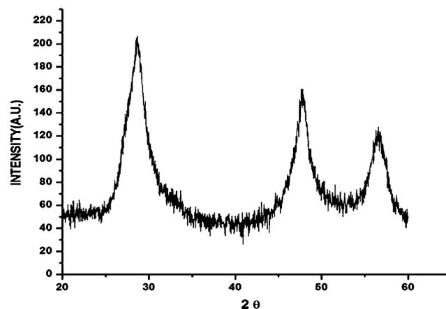
Fig. 2 XRD patterns of ZnS nanoparticles.
