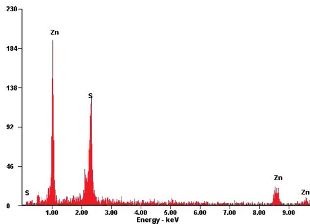
Fig. 5 EDAX pattern of ZnS nanoparticles (after use as catalyst).
