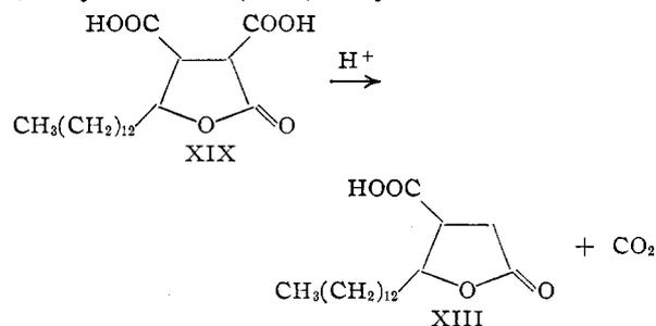
physical character of the salt, the free diacid was an unmanageable, amorphous substance. The assignment of structure was confirmed by acid-catalyzed decarboxylation, which yielded the previously obtained carboxylactone XIII.
