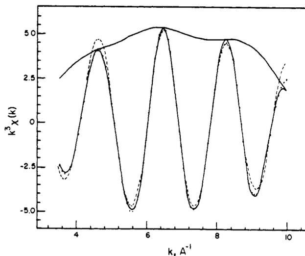
**Figure 1.** Fourier transform (a) and filtered data (b) of the  $k^3\chi(k)$  vs  $k$  EXAFS spectrum from the nickel edge of CO dehydrogenase. The upper curve in (a) is the window function used in Fourier filtering. The dashed line in (b) is the one term sulfur fit to the Fourier filtered data (solid line) while the dotted line is the fit of one sulfur plus iron. The amplitude function for the filtered data is also shown.
