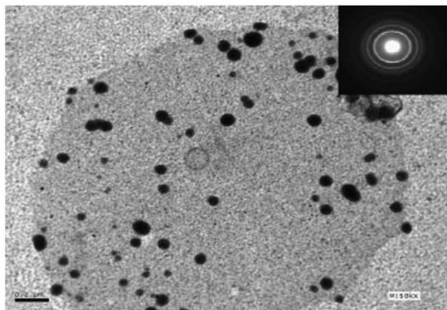
FIG. 2. TEM of the reduced silver nanoparticles.
