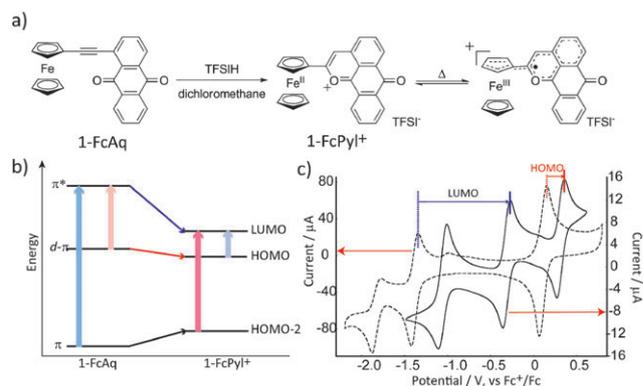
**Fig. 1** Protonation-induced cyclocondensation of 1-FcAq to produce 1-FcPyl<sup>+</sup> and the valence tautomerization of 1-FcPyl<sup>+</sup>. (a) Changes in the chemical structure. (b) Energy diagram for 1-FcAq and 1-FcPyl<sup>+</sup>. (c) Cyclic voltammograms of 1-FcAq (dotted line) and 1-FcPyl<sup>+</sup>TFSI<sup>−</sup> (solid line) in 0.1 M Bu<sub>4</sub>NClO<sub>4</sub>–CH<sub>2</sub>Cl<sub>2</sub> at 0.1 V s<sup>−1</sup>.
