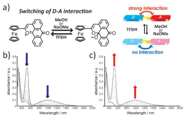
**Fig. 4** Alcohol and acid responses of 1-FcPyl<sup>+</sup>. (a) Switching of the D–A interaction between 1-FcPyl<sup>+</sup> and 1-FcPyl-OMe. (b) UV-Vis–NIR spectral changes in 1-FcPyl<sup>+</sup> upon the addition of 0 (solid line) to 80 μL methanol (dashed line). (c) UV-Vis–NIR spectral changes in 1-FcPyl-OMe upon the addition of 0 (solid line) to 1 eq. of TFSIH (dashed line).
