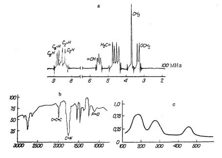
Fig. 1. a) PMR, b) IR, and c) UV spectrum of inosine dialdehyde 9-(morpholyl-3'-hydroxy-4'-methyl-5'-propadienephosphinate-6'-hydroxymethyl-2')-hypoxanthine (I). On the abscissa axis is shown a) the chemical shift (in ppm), b) wavenumber (in cm<sup>-1</sup>), and c) wavelength (nm); and on the ordinate b) transmission (%), and c) optimal density (in relative units).
