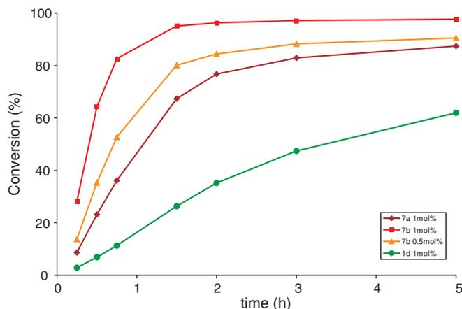
Fig. 4. Activity of **1d**, **7a** and **7b** in RCM of **10a** in dichloromethane, 26 °C, 5 h; conversions according to GC.
