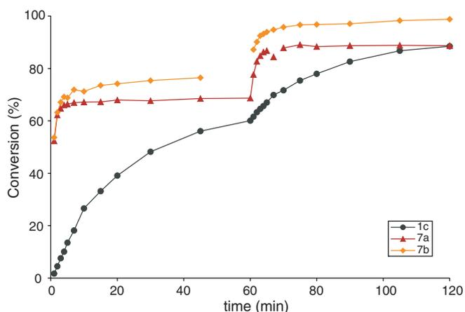
Fig. 5. Activity of **1c**, **7a** and **7b** in RCM of **12** in toluene, 80 °C, 2 h; catalysts were added in two portions (0.4 + 0.2 mol% Ru). Conversions according to HPLC.
