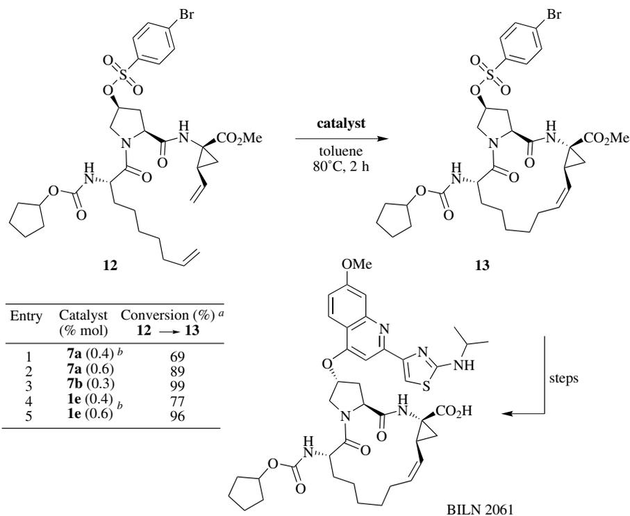
Scheme 4. Comparative study of catalysts **1e**, **7a** and **7b** activity in cyclization of BILN 2061 precursor **12**. Reaction conditions: 0.3–0.6 mol% of catalyst, toluene, 80 °C, 2 h. <sup>a</sup> Conversion determined by HPLC after 2 h. <sup>b</sup> Conversion determined by HPLC after 1 h.
