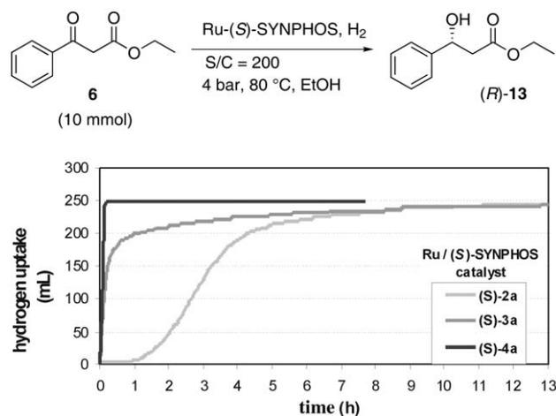
**Figure 2** Kinetics of hydrogen uptake in asymmetric hydrogenation of substrate **6** using Ru-SYNPHOS catalysts (*S*)-**2a** (ee = 91.9%), (*S*)-**3a** (ee = 94.2%) and (*S*)-**4a** (ee = 98.3%).
