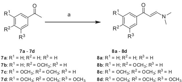
**Scheme 1.** Synthesis of the enaminones **8a–8d**. Reagents and conditions: (a) DMF-DMA, 150 °C, 20–30 h.
