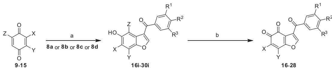
**Scheme 2.** Synthesis of benzofuran-4,5-diones. Reagents and conditions: (a) AcOH, rt; (b) For **16**, **17**, **19**, **21**, **28**: Dess–Martin periodinane, DMSO, 0 °C–rt, 20 min; For **5**, **20**, **22–27**: HNO<sub>3</sub>, AcOH, rt→65 °C, 3 h. Z = Br or Cl, matching X and Y.
