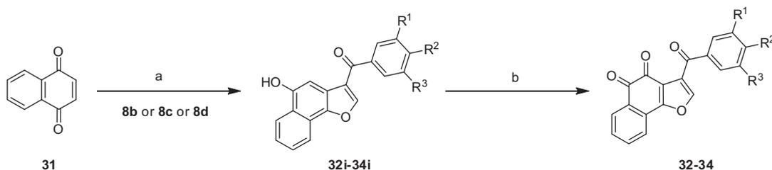
**Scheme 3.** Synthesis of naphthofurandiones. Reagents and conditions: (a) AcOH, rt; (b) HNO<sub>3</sub>, AcOH, rt→50 °C, 30 min.
