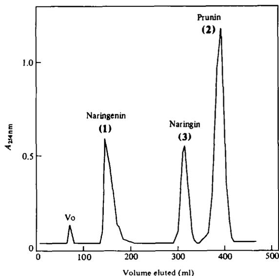
Fig. 1. A typical separation of authentic flavonoids using a  $2.5 \times 100$  cm BioGel-P4 column. Flow rate was 20 ml/hr. A 5 mM solution of  $(\text{NH}_4)\text{HCO}_3$  pH = 7.8 was used as eluant. Note the high resolution of the separation.
