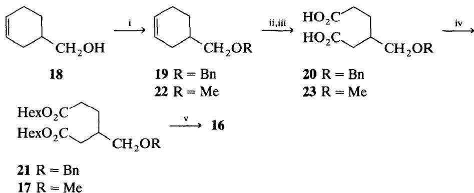
*Reagents:* (i) RHal/NaH/(CH<sub>2</sub>OMe)<sub>2</sub>; (ii) O<sub>3</sub>/O<sub>2</sub>-MeOH; (iii) H<sub>2</sub>O<sub>2</sub>/H<sub>3</sub>O<sup>+</sup>;
