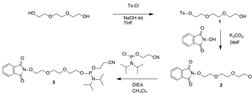
Scheme 1. Synthesis of phthalimideoxy-triethyleneglycol phosphoramidite **3**.
