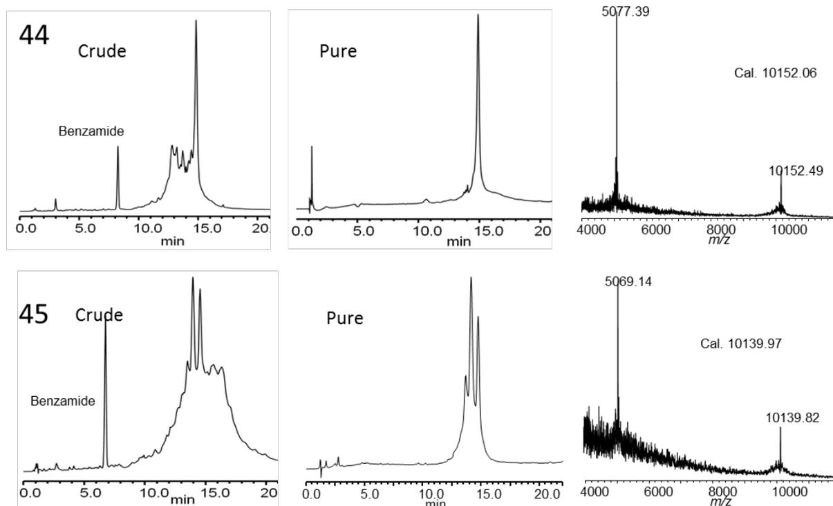
Figure 4. HPLC profiles and MALDI-TOF MS of (top) acetone-capped linear oligonucleotide **44** and (bottom) bicyclic oligonucleotide **45**.
