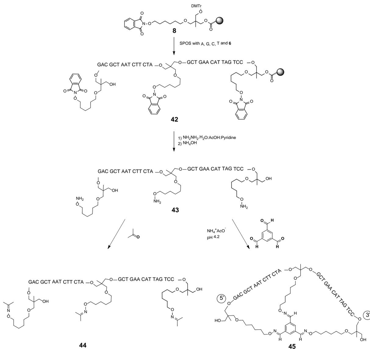
Scheme 8. Synthesis of a bicyclic oligonucleotide
